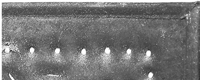
Very uniform, and with precise corners, the edges of the door on this lantern suggest 19th century machine use.
