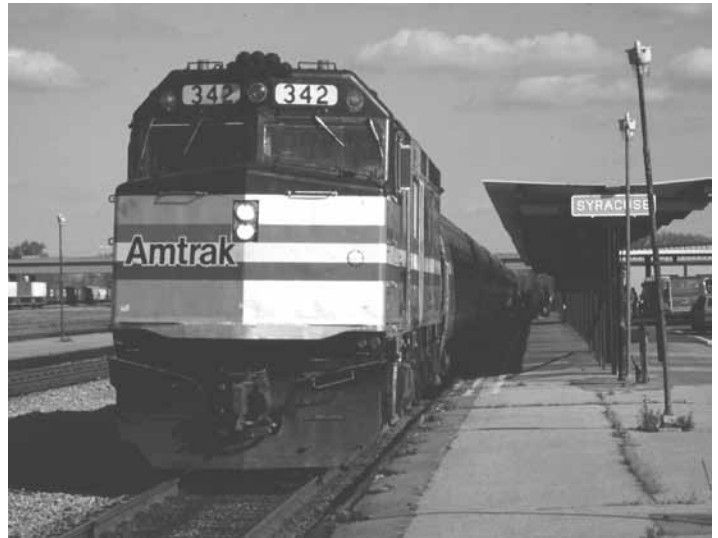
The F40PH locomotive, which pulled Amtrak trains for almost 30 years, used the Nathan P1234A5 on the first order, and the Nathan KL5A horn on subsequent models.
