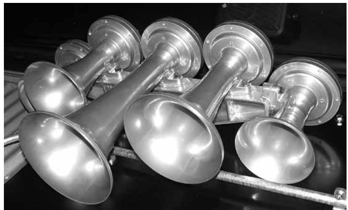
The Nathan Airchime K5LA horn is now standard on all locomotives, and has become the new "sound of Amtrak."
