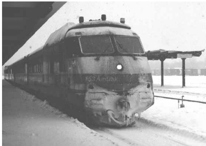
Amtrak's Rohr turboliner trainsets were equipped with Nathan Airchime model P1234A5 air horns.
