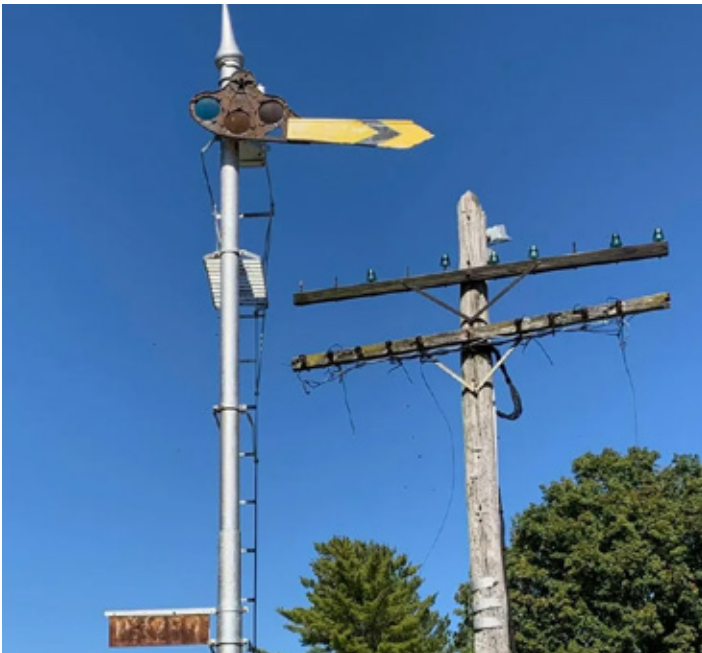
A $1550 bid was needed to buy this complete General Railway Signal 2A semaphore signal from the Monon.
