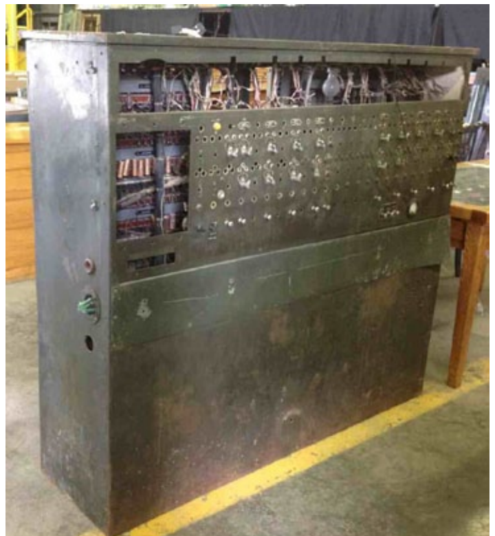
One of the many unique items in the sale, the original CTC machine from the NYO&W, later used on the Western Maryland Railroad, sold for a reasonable $375.
